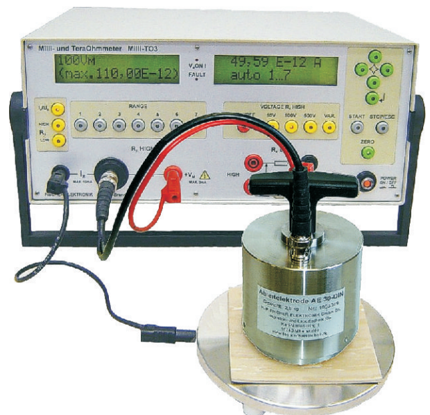
surface measurement with AE 30-DIN and grounded base plate GP 14 (optional) connected to Milli-TO 3
