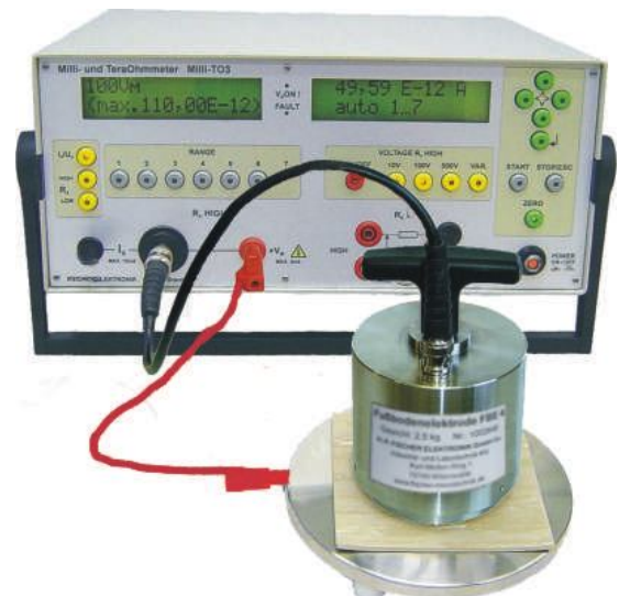
Volume resistance measurement with FBE 4 and earth plate GP 14 * and Milli-TO 3 *
