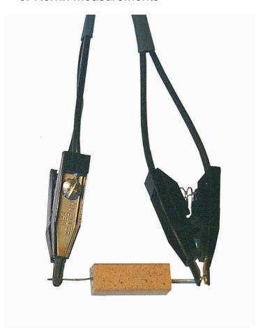
The Kelvin Clamp KEZ-Mini 1 is a four-wire clamps pair for the measurement of low resistances at specimen with small dimensions.
